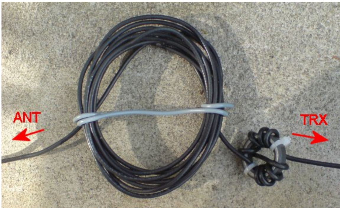
Coiled coax at antenna side of choke
